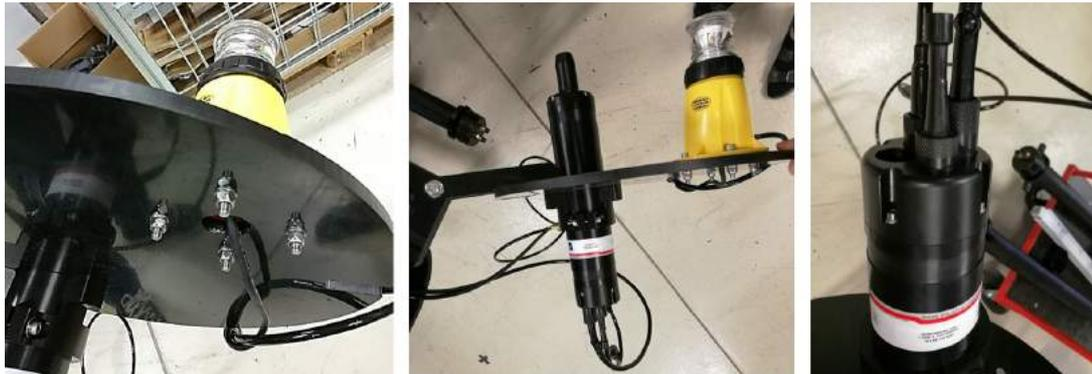
Picture 1: a) Blinking light mounting, b) AOS tube mounting, c) Output AOS tube
