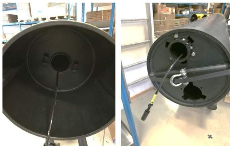
Picture 2: Pull the cable(s) through the buoy. a) seen from top of buoy: cable pulled through buoy. b) seen from bottom of buoy: cable pulled through buoy.
