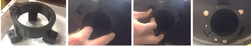
Picture 3: a) Clamp for Aquadopp Profiler. b) Place the bracket in the slot. c) Adjust and align the clamp with the holes in buoy. d) Use the supplied screws for fastening
