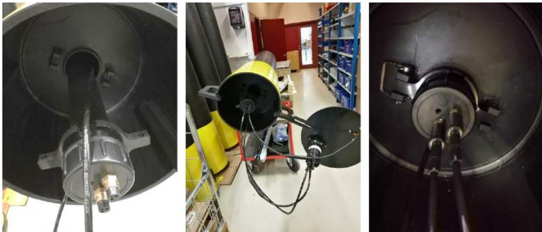
Picture 5: a) Place the cables in the indent of the battery tube collar. b) Mount the cable from the AOS tube and the cable from the blinking light to the battery tube. c) Use the supplied locking splints to fasten the
