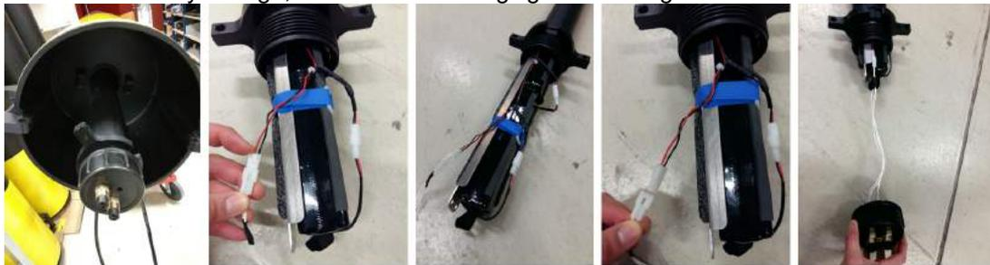
Picture 1 a) Open top cover and drag out battery tube. b) loosen the white molex-connector. c) Take out the battery rail. Note the placement of the batteries. Replace with new batteries d) Connect the molex-contact. e) tighten the battery cover.
